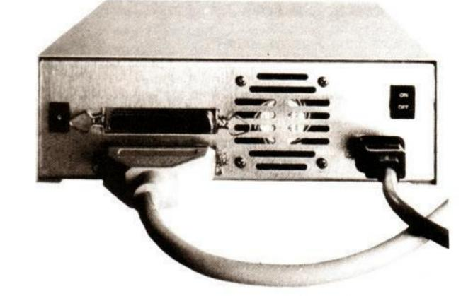
BAIL MOUNTS TO SECURE YOUR CABLES TO THE DRIVE EASY ACCESS TERMINATOR REMOVAL FOR DAISY CHAINING
