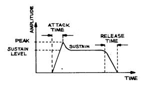
So the four parts of our basic amplitude envelope are attack time, decay time, sustain level (the volume at which a sound sustains, if it sustains) and release time. The common abbreviation is ADSR. RCORROWS17
