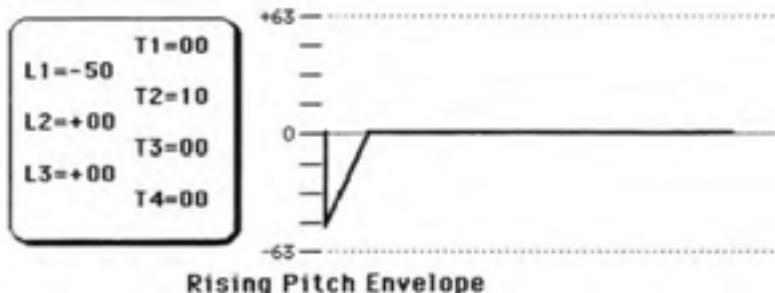
This could be a rather long, dramatic "slide", or an almost imperceptibly short one, depending on the value you assign to TIME 2. How much the Pitch is altered will depend on the value of LEVEL 1 and the Modulation depth.
