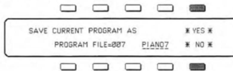
The data will be saved to the lowest-numbered empty Single-Program block on the disk. The lower-left portion of the Display (FILE=\_\_\_\_) shows you which of the 128 Single-Program blocks the data will occupy on the disk.
