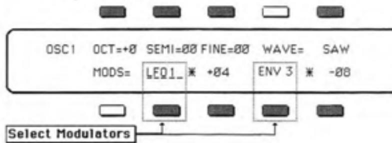
For Modulating Program **Pan** [**DCA 4** Page] and LFO depth [**LFO UFO 2** and **LFO 3** Pages] only one Modulator can be selected.
