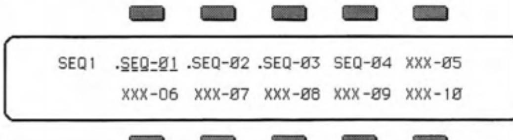
Press the SEQ button again. Now pressing these same three Bank Select buttons will show you the **Sequence Select Pages** for the next three Sequencer Banks, numbered **SEQ 4**, **SEQ 5** and **SEQ 6**. These Sequences are numbered 31 through 60.
