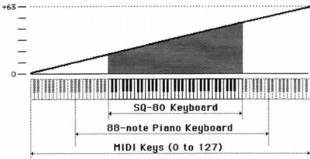
Modulation depth will reverse the effect). Since scaling starts from MIDI key 0, there will always be some effect on the **SQ-80** keyboard, even on the lowest note. Manual Levels should be adjusted accordingly.
