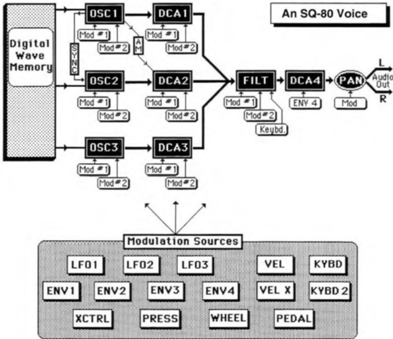
Any of 'these 15 Modulation Sources can be independently assigned wherever a MOD is indicated above.'
