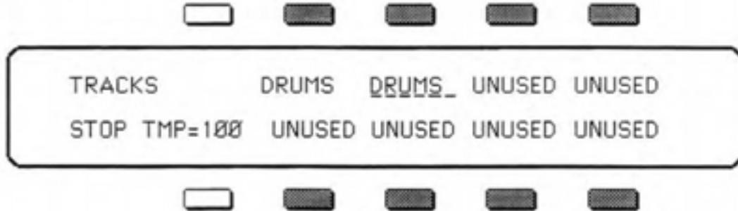
The Program from Track 1 was "carried over" and assigned to Track 2 when it was selected. **Selecting an UNUSED Track automatically assigns that Track the Program, and all the Mix'MIDI Data, from the previously selected Track (or the "Straight Synth" Program and MIDI Channel, if no Track was selected).**
