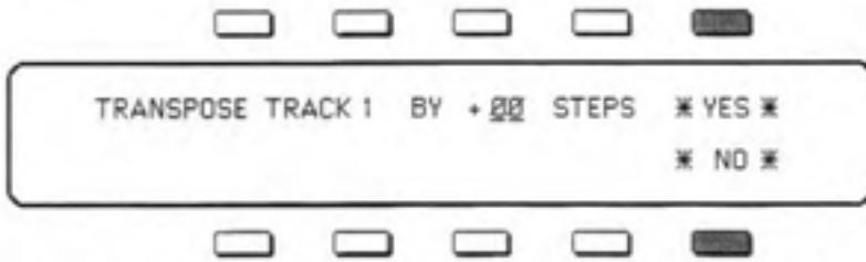
One Step is a half-tone (up or down by one key); four Steps, a major third; seven Steps, a fifth, and so on. Range is from -12 (Down one Octave) To +12 (Up one Octave).
