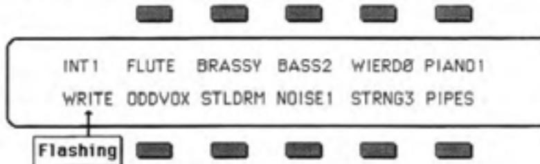
When you release the Bank Select Button, the Display will return to the **WRITE PROGRAM Page**. Press another Bank Select Button and the Display shows you the Programs for that Bank. To look at the Programs in a different Master Bank (CART A or **CART B** for instance), simply press the Button for that Master Bank, and then press and hold down any of the four Bank Select Buttons, as before.
