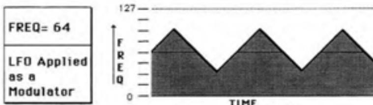
Of course, since two Modulators can be selected, you could apply both of these Modulators (or any other combination) to the Filter Cutoff Frequency, and their effect would be added together, and then added to the Manual Level.
