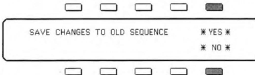
**Pressing \*YES\*** saves the Sequence, with the current settings of all the parameters listed above, into Sequencer Memory.
