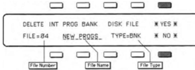
DISK DRIVE..." and then returns to the **Storage** Page. The file is Deleted and the Program Bank block it occupied on the disk is now available.
