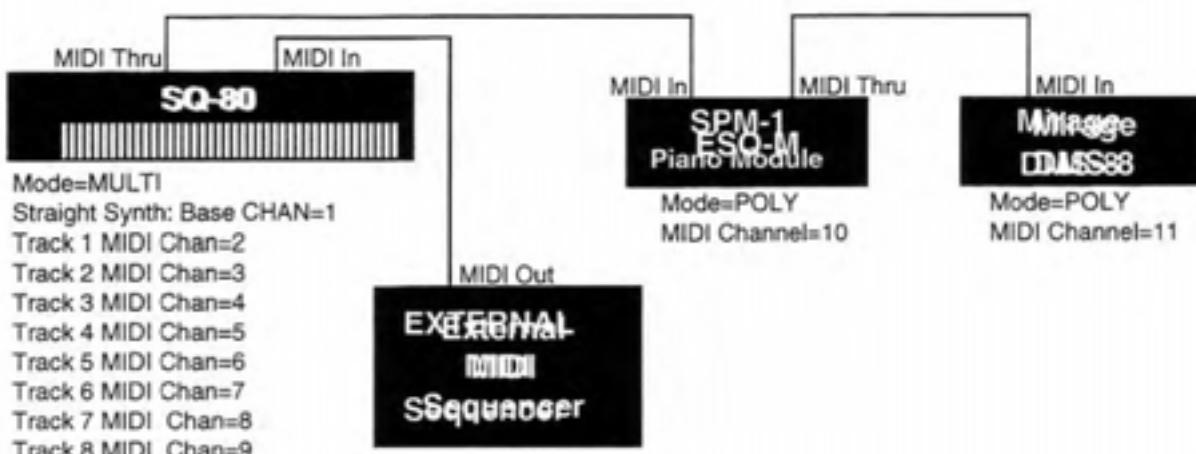
As you can see, the set-up is similar to the earlier POLY Mode example, except that now the SQ-80 is responding to nine MIDI Channels rather than one. The ESQ-M and the **Mirage** have been set to receive on MIDI Channels 10 and 11 respectively.
