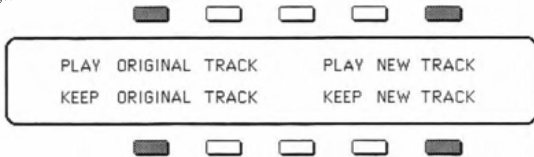
You can now audition the Quantized Track, to see if the effect was what you wanted. Play the new (Quantized) Track, or the Original (Unquantized) Track, pressing Stop'Cont to halt the Sequencer between plays. The **Auto-Locate** Controls on the LOCATE Page can be used before either PLAY command, to start from somewhere other than the beginning of the Sequence.
