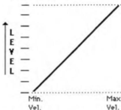
**From 00X to 63X, LV causes Envelope levels to increase exponentially — little effect until maximum velocity.**
