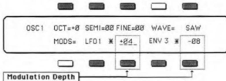
**Helpful Hint:** With Modulation Depth, as with all Parameter values that have a center value (in this case, **+00**), there is an easy way to reach that value. With the Modulation Depth selected, press the Down Arrow Button, and while holding it down, press the Up Arrow Button. This automatically sets the Modulation Depth to **+00**.
