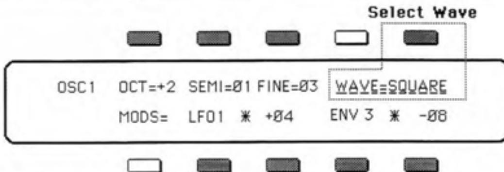
Press the "Soft" Button above the **WAVE NAME**. Now you can use the Data Entry Slider and the Up and Down Arrow Buttons to change the Wave that **OSC 1** will play. There are 75 available choices, each with its own Name. Follow the same procedure to select a Wave for **OSC 2** and **OSC 3**. The following section details each Wave by Name.
