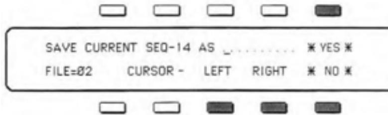
The data will be saved to the lowest-numbered empty Sequencer/Sys-Ex Block on the disk. The lower-left portion of the Display (FILE=\_) shows you which of the ten Sequencer/Sys-Ex Blocks the data will occupy on the disk.
