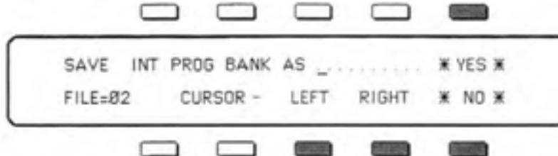
The data will be saved to the lowest-numbered empty Program Bank File on the disk. The lower-left portion of the Display (FILE=\_ ) shows you which of the forty Program Bank blocks the data will occupy on the disk,
