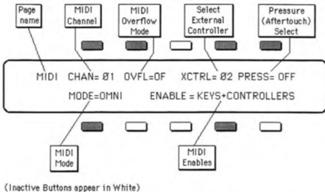
From this Page you control the MIDI (Musical Instrument Digital Interface) configuration of the SQ-80 as well as determining which type of Pressure the **SQ-80** keyboard will generate locally and send out via MIDI. Because of its built-in Sequencer, its controller-oriented features and its ability to receive and store System Exclusive information from any MIDI instrument, the SQ-80's MIDI implementation is a bit more involved than most synthesizers.
