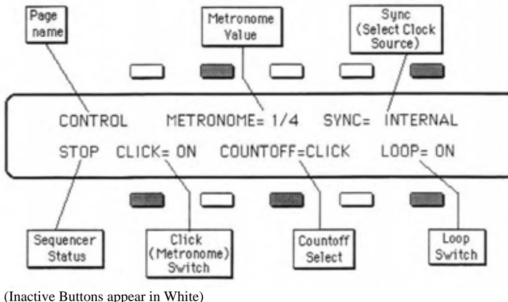
Before recording or playing back a Sequence, you will want to select the **CONTROL** Page and adjust its parameters to suit your current needs. From this Page you control the CLICK track (or metronome), the COUNTOFF (a one measure count, with or without Click track, before the Sequence begins), the LOOP switch and the Clock Source.
