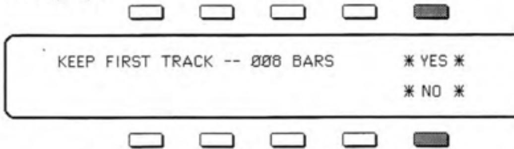
**Pressing \*YES\*** installs the Track in Memory as the First Track of the Sequence, and defines the length of the Sequence as the number of Bars shown.
