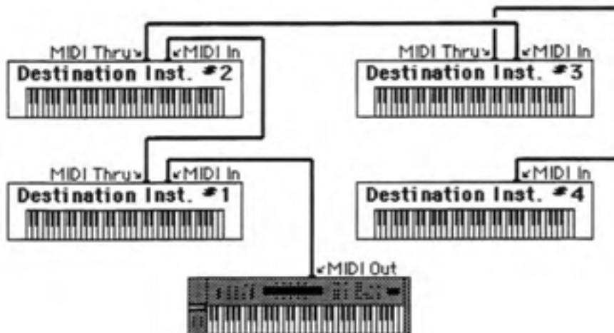
If one (or more) of the receiving devices has a single MIDI Jack which is switchable between **MIDI Out** and **MIDI Thru**, be sure to set that instrument for **MIDI Thru**. Or make it the last one in the chain.
