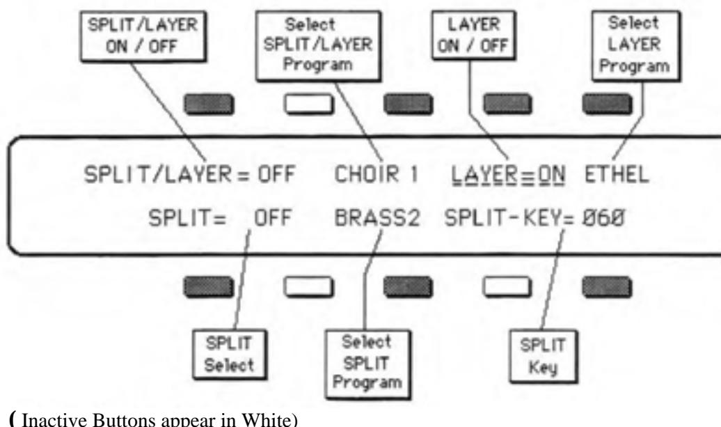
Programs on the SQ-80 can be Layered (so that two Programs play at once over the whole keyboard), **Split** (so that each half of the keyboard plays a different Program), and **Split/Layered** (so that the **Split** Program is layered with yet another Program).
