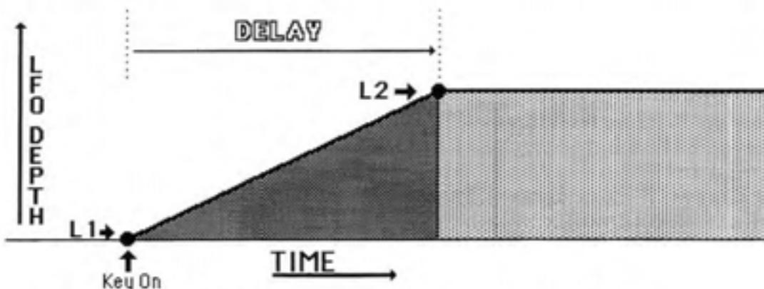
**Example of LFO Modulation which 'fades in' over Time.**
