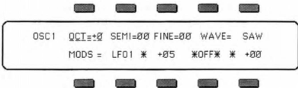
In the top left-hand corner of the Display you will always find the Name of the Page, which corresponds to that of the button you pressed. To the right of that are the various parameters which can be selected and modified from this page.
