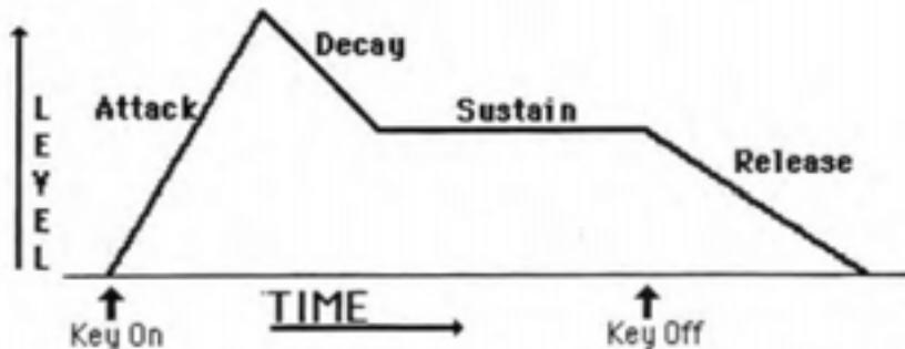
Notice that an Envelope is really just a series of Levels that change through Time. With the four parameters of the ADSR Envelope, we can control three Times (Attack, Decay and Release) and one Level (Sustain). This is fine for many basic volume and brightness Envelopes, but for more complex sounds — for subtle pitch Envelopes and other cool effects — it becomes necessary to have more specific control over more **Times** and **Levels**. Which brings us back to the SQ-80.
