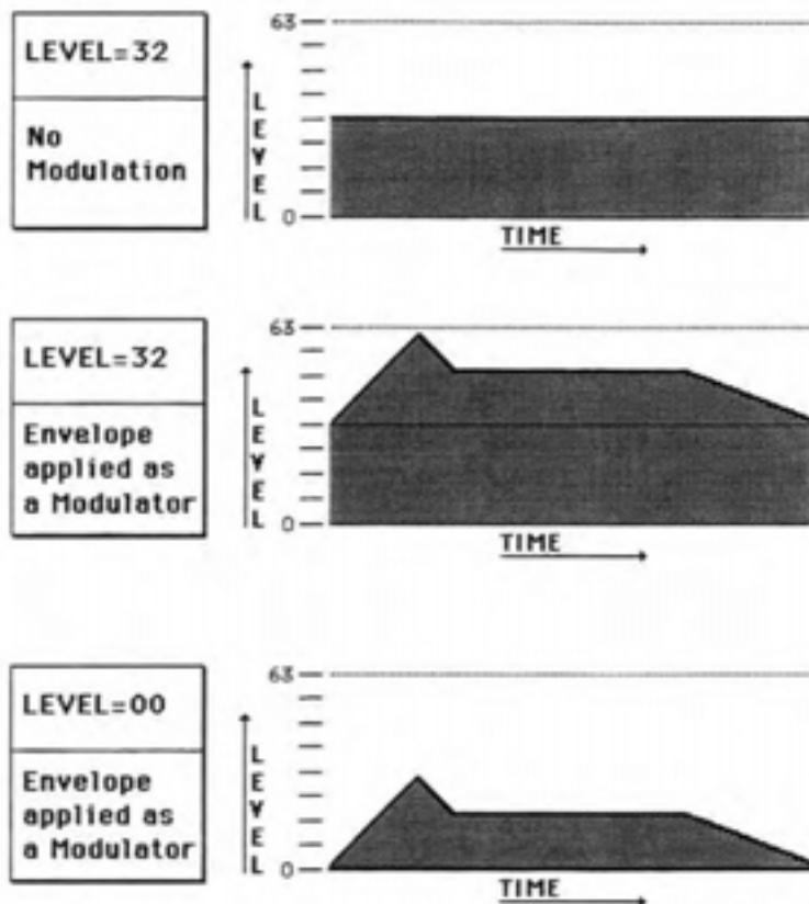
This last combination (LEVEL=00, Envelope selected as a modulator, modulation depth greater than Zero) is the best way to "fade in" the Oscillator(s) playing the Sustain portion of a sound when a Transient Attack Wave is being played by another Oscillator. Usually we use ENV 2 for this purpose. Set the Envelope's TIME 1 to a value around 10. This will cause the volume of the Sustain Wave to fade in as the Transient Attack Wave fades out.
