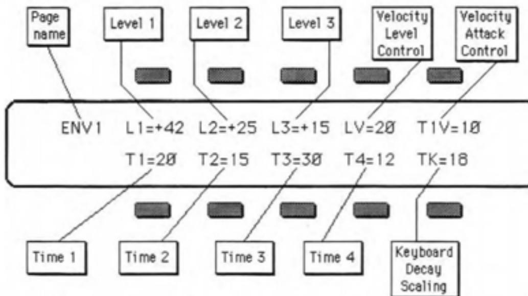
The format of the **Envelope** Page is the same for **[ENV 1]**, **[ENV 2]**, **[ENV 3]** and **[ENV 4]**, although each Page is independent. The Envelopes are used as Modulators, and may be applied wherever a Modulation Source is selected.
