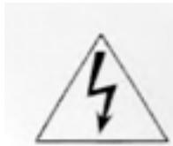
This symbol is intended to alert the user to the presence of uninsulated "dangerous voltage" within the product's enclosure that may be of sufficient magnitude to constitute a risk of electronic shock to Persons.
