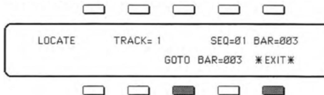
—> Use Data Entry Slider and the Up and Down Arrow Buttons to adjust the **GOTO** Bar number to the Bar at which you want to start. You can choose any Bar within the current Sequence.
