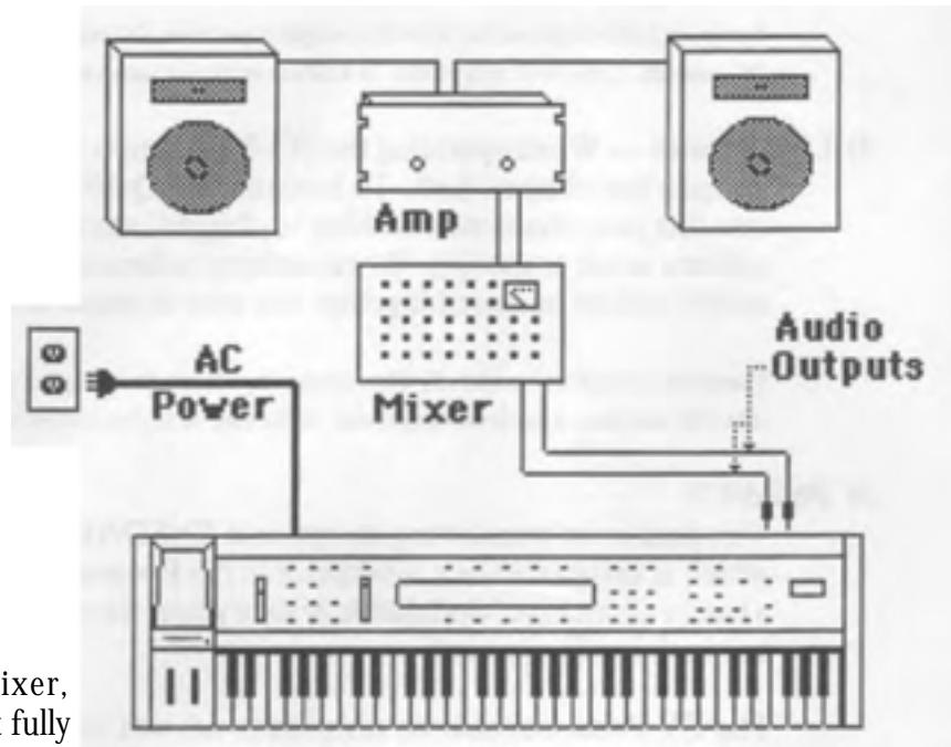
**Note:** The **SQ-80**'s outputs are line-level and are intended to be connected only to line-level inputs such as those on a mixer, stereo pre-amp, keyboard amp, etc. Connecting the SQ-80's audio outputs to a midlevel input, such as a guitar amp or the microphone jacks on a tape deck, is not recommended.
