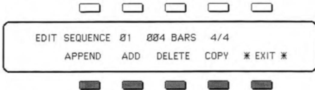
The upper portion of the Display tells you which Sequence is selected, how many Bars long that Sequence is, and its Time Signature. As with all **EDIT** Pages, the **EXIT** Button is there in the lower-right corner, so you can bail out at any time. Pressing **EXIT** will return you to the **EDIT** Page.
