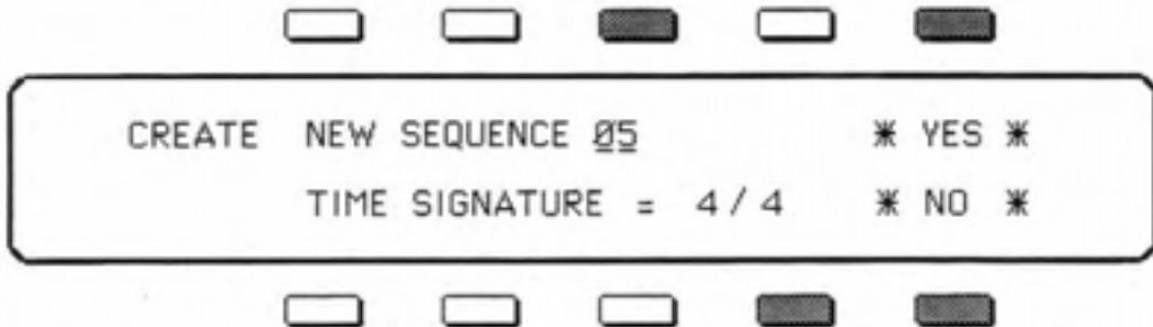
—> **Select a Memory Location.** Use the Data Entry Slider and the Up and Down Arrow Buttons to select which Sequence Memory Location you wish to create the new Sequence in. Only the numbers of empty, or undefined, Locations are available for selection.
