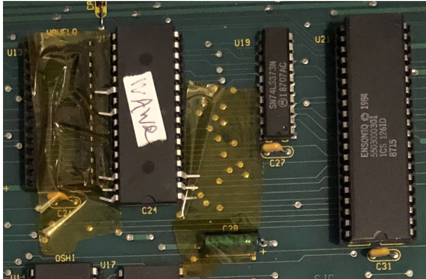
Figure 2 - from left to right: Wave ROM, 73LS373 IC (U19), Ensoniq DOC sound IC (U21)
